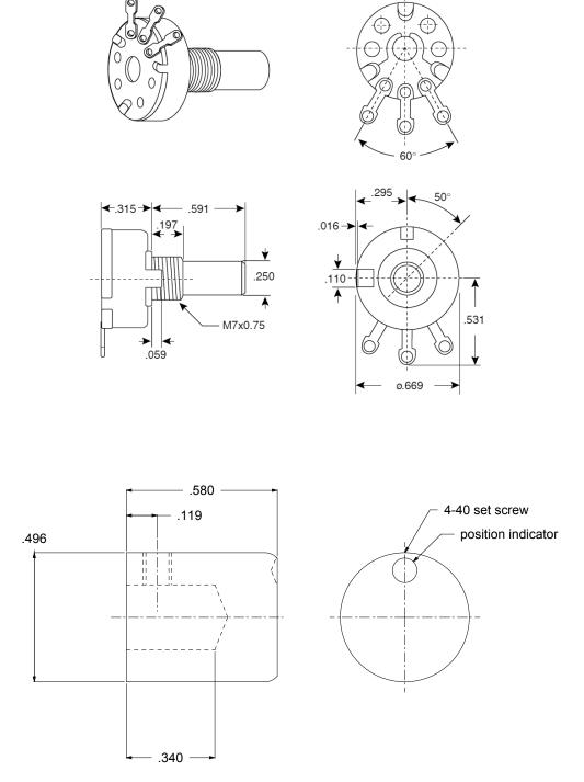
Leads are 3.440" long stranded 22 gauge with TFE insulation. 1k resistance.
