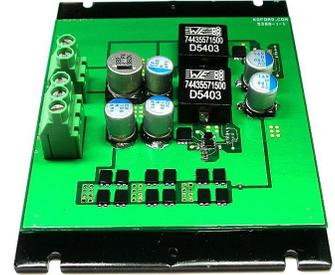
Absolute maximum input voltage from motor 40V. Output current is internally limited to 20 amps. Output is short circuit protected. Minimum voltage drop at 15 amps = .209V. Connections by terminal blocks. Motor leads connect to A, B, C, output leads connect to + and -
