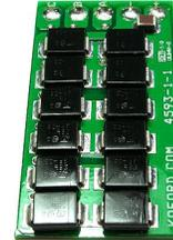
Absolute maximum voltage 40V. Absolute maximum output current 8 amps. Voltage drop at 6 amps .8V. Connection to circuit by soldering to pads. Motor leads solder to A, B, C, output leads solder to + and -, weight .4 oz.
